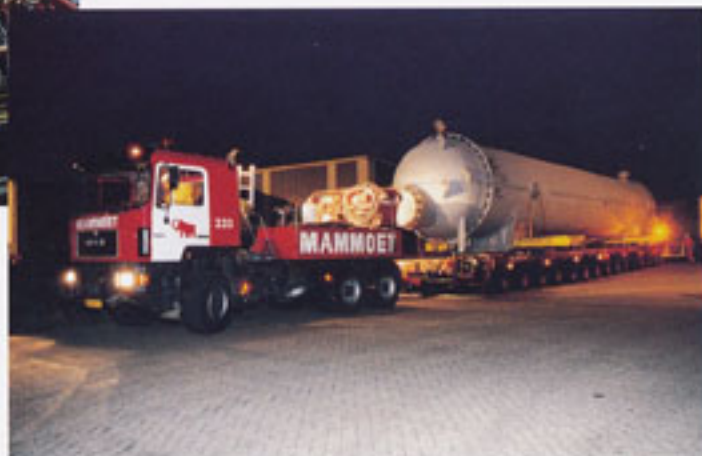
Dunkerque/Geleen - A 240 tonne pool reactor and other equipment were transported from the factory in France to the DSM chemical plant in Geleen over land and by water. At the Urea plant UF2 FSM Geleen project, Mammoet's 400 tonne lattice boom crane with superlift attachment took care of the lifting and positioning.
