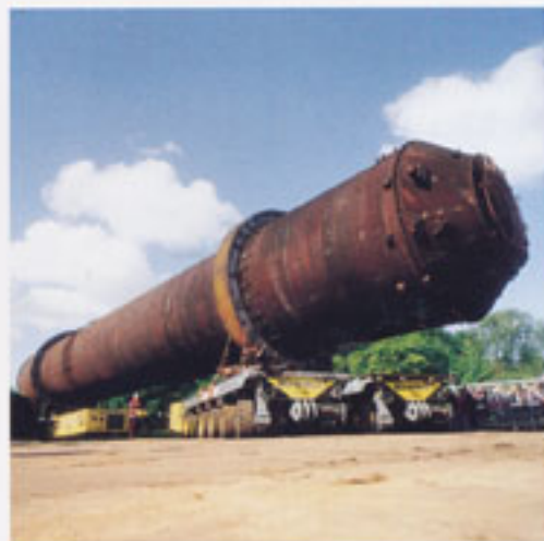
Klazienaveen - A spectacular movement of a so-called rotating furnace was performed by Mammoet's SPMTs which attracted a lot of attention from the neighbourhood. The 450 tonne furnace had a diameter of 4.5 metres and a length of 36 metres. An additional difficulty was the fragile fireproof brickwork inside the oven which was not allowed to break loose.
